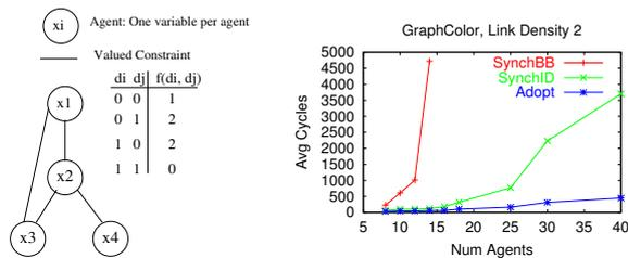
**Figure 8:** (a) An example DCOP with four agents. Agents must choose values for their respective variables to minimize the sum cost over all valued constraints. (b) The Adopt algorithm for DCOP significantly outperforms synchronous methods on benchmark problems.
