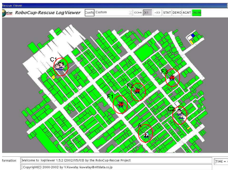
Figure 3: RoboCupRescue Scenario: C1 and C2 denote the two fire locations, F1, F2 and F3 denote fire stations 1, 2 and 3 respectively and A denotes the ambulance center.
